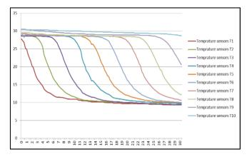
Figure 8. Thermocline for a flow rate of 200 ltr/hr
