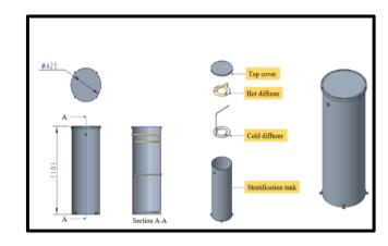
**Figure 2.** Mechanical architecture of stratification tank (All dimensions are in mm)
