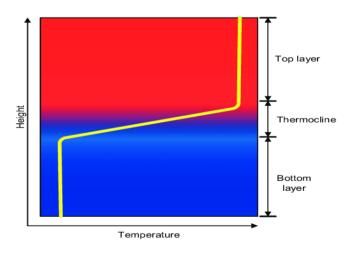
**Figure 4.** Thermocline in storage tank
