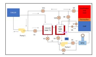
Figure 1. Schematic diagram of TES by stratification
