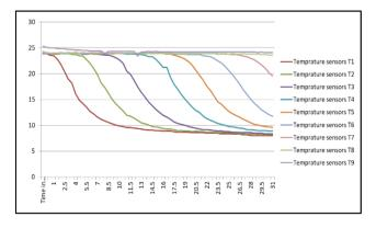
Figure 7. Thermocline for a flow rate of 150 ltr/hr
