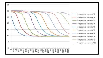
Figure 6. Thermocline for a flow rate of 100 ltr/hr
