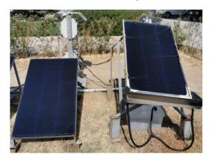
Figure 2. Photovoltaic panels experimental rig
