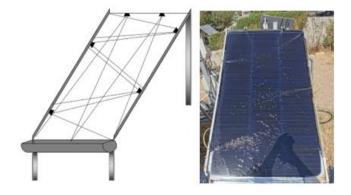
**Figure 3.** Schematic diagram and experimental rig of nozzles location over the panel
