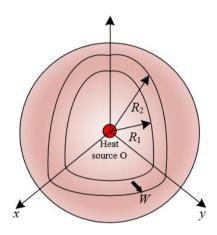
**Figure 3.** Schematic diagram of isothermal surfaces of the point heat source of the rock mountain
