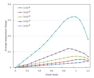
**Figure 5.** Change of average temperature with axial strain in the rock model under different thermal expansion coefficients
