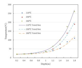
**Figure 7.** Temperature and depth relationship curve of the rock mountain under steady-state heat conduction
