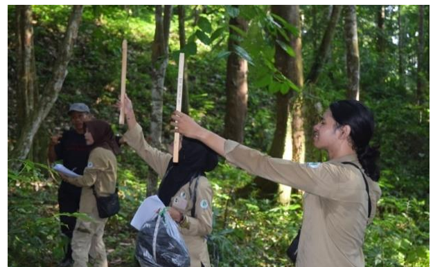
Figure 4. Measure the height of the tree with a Christian Hipsometer
