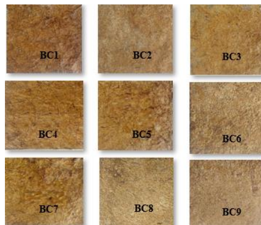
Figure 3. The physic of SCB/CF hybrid bio-panels (a) BC1, (b) BC2, (c) BC3, (d) BC4, (e) BC5, (f) BC6, (g) BC7, (h) BC8, (i) BC9
