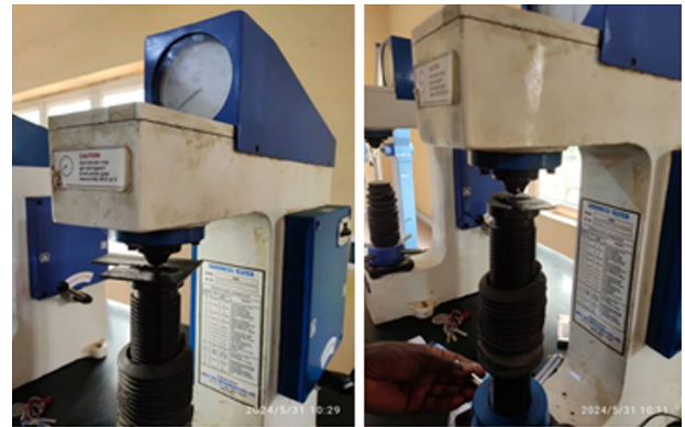
Figure 11. Hardness testing of welded joint
