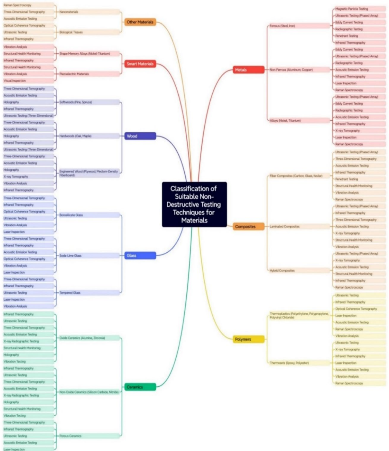
Figure 7. Graphic mind map representing a classification of techniques adapted to different types of materials
