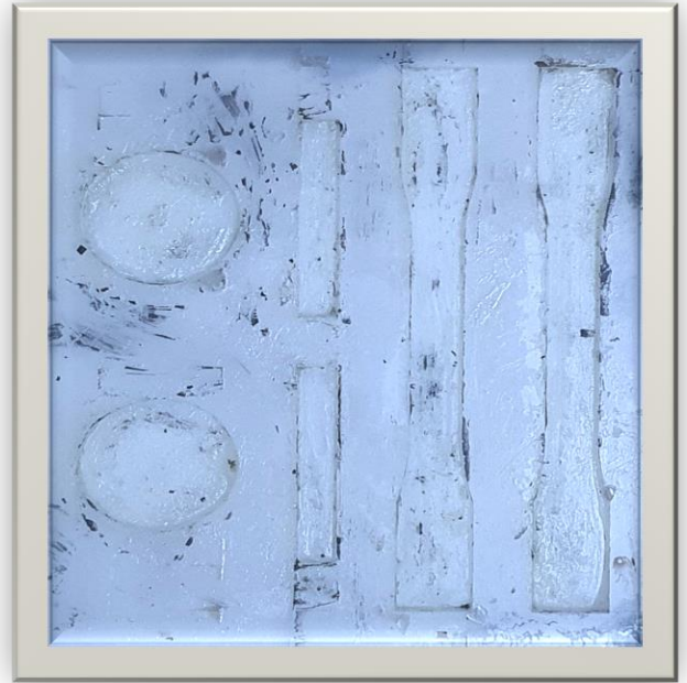
Figure 1. Silicon mould for preparing samples
