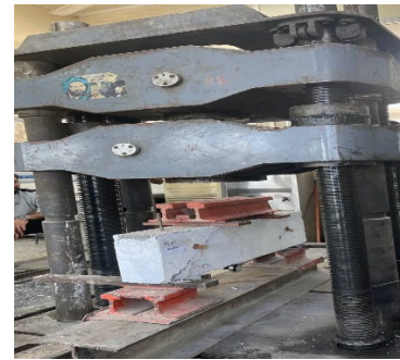
Figure 2. Deep beam test under a symmetrical point load
