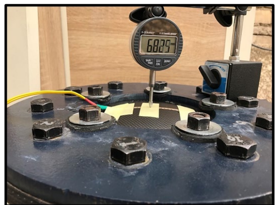
Figure 6. CFRP specimen under 5 \times 10^5 N/m 2 distributed compression test
