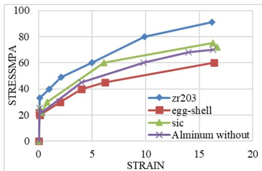
Figure 12. Stress-strain before shot peening
