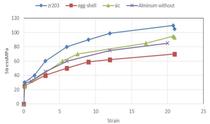
Figure 13. Stress-strain after shot peening (5 min)
