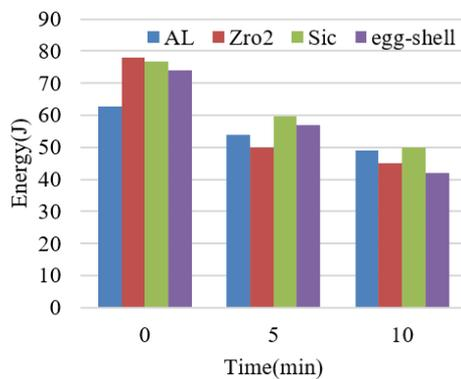
Figure 16. Comparison energy with and without shot peening
