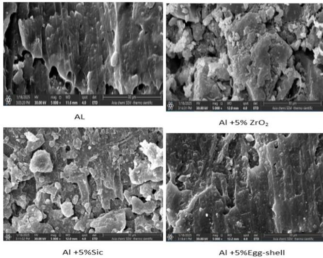
**Figure 8.** Microstructure for samples with different addition
