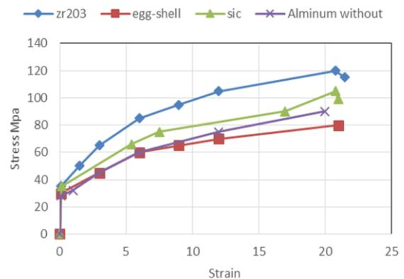
Figure 14. Stress-strain after shot peening (10 min)
