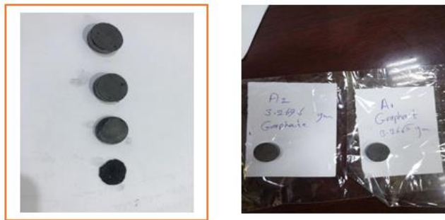
Figure 7. Photos of graphite-carbon soot composite anode
