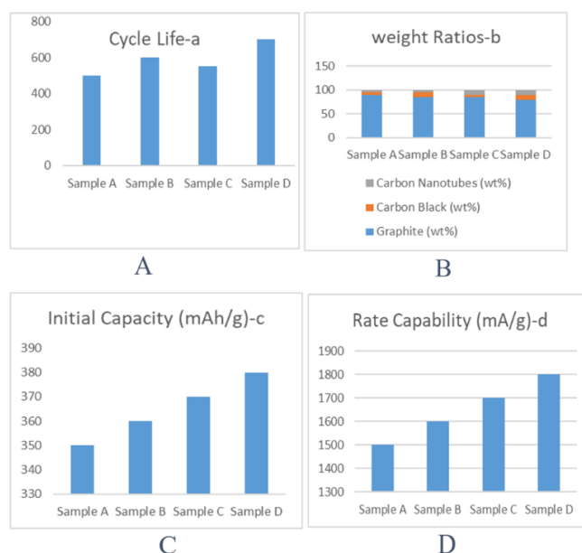
Figure 11. Electrochemical test due to (A-D) composite anode half cell model LIB
