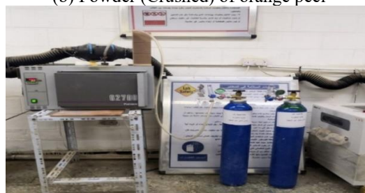
(c) Carbonization with N 2 gas and Activation with CO 2 gas
