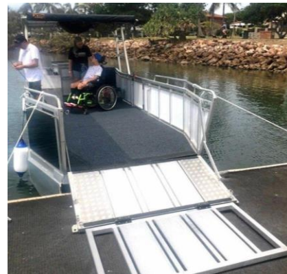
Figure 7. Anti slip deck and ramp for wheelchair users [42]
