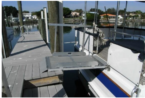
Figure 5. Ramp for access point wheelchair [34]
