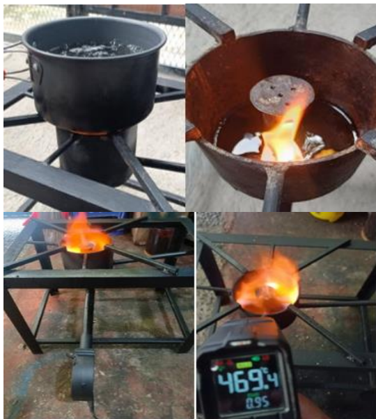
Figure 7. Trial of prototype cooking stove using maggot BSF oil fuel
