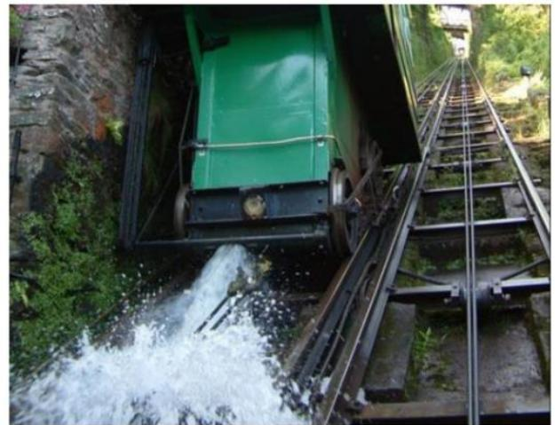
Figure 2. The Lynton and Lynmouth Cliff Railway car operates without electrical power and fuel [4]
