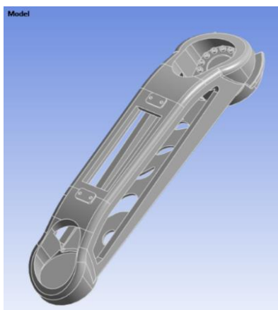
Figure 12. The robot's upper arm after topology optimization
