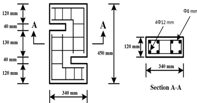
**Figure 1.** Dimensions of the DSSs and steel reinforcement details
