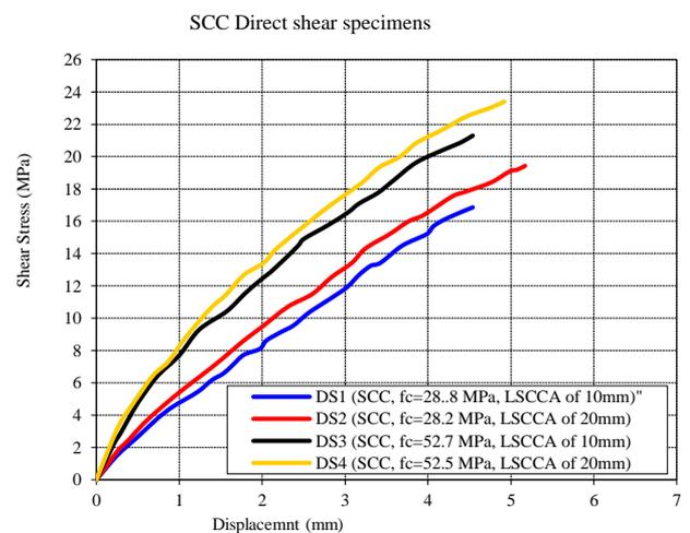
**Figure 6.** Shear stress-displacement relationship of SCC-DSSs
