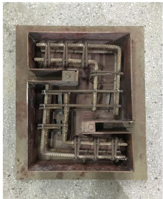
**Figure 2.** Steel reinforcement details of the DSSs
