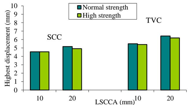
**Figure 5.** Highest displacement of SCC and TVC DSSs
