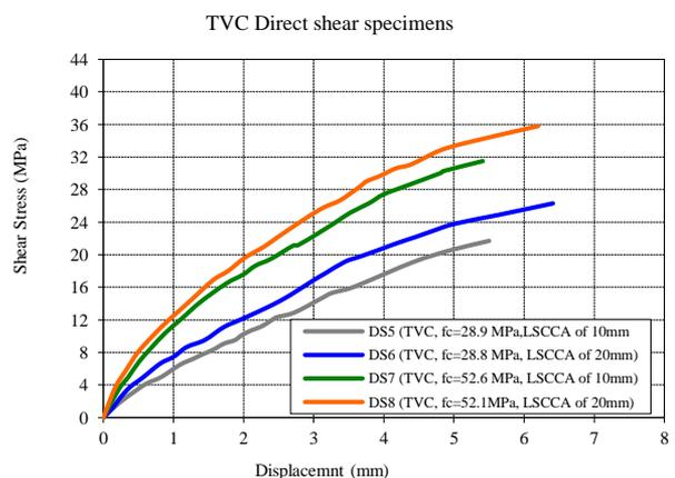
**Figure 7.** Shear stress-displacement relationship of TVC-DSSs
