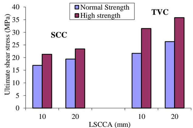
**Figure 4.** Ultimate shear stress of SCC and TVC DSSs
