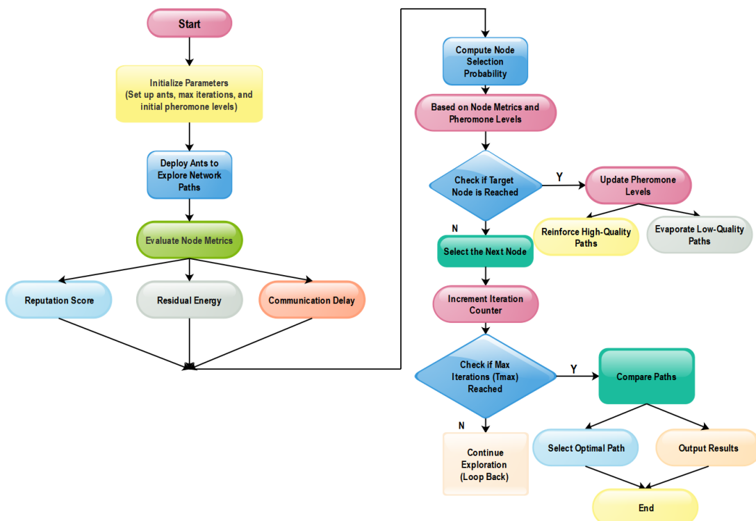
Figure 8. The proposed optimal wireless sensor network ant-lifetime routing algorithm using multi-phase pheromone
