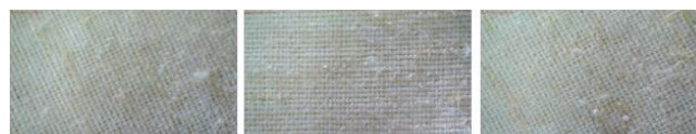
Figure 3. Photos of pilling formation on woven fabric from bamboo fiber blended with recycled polyester after 30 minutes
