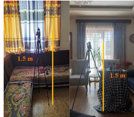
Figure 6. The equipment position inside the living room in casus study
