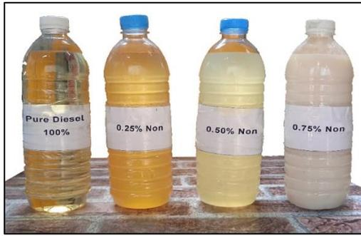
**Figure 3.** a) Pure diesel; b) 0.25% Al<sub>2</sub>O<sub>3</sub>+Di; c) 0.50% Al<sub>2</sub>O<sub>3</sub>+Di; d) 0.75% Al<sub>2</sub>O<sub>3</sub>+Di
