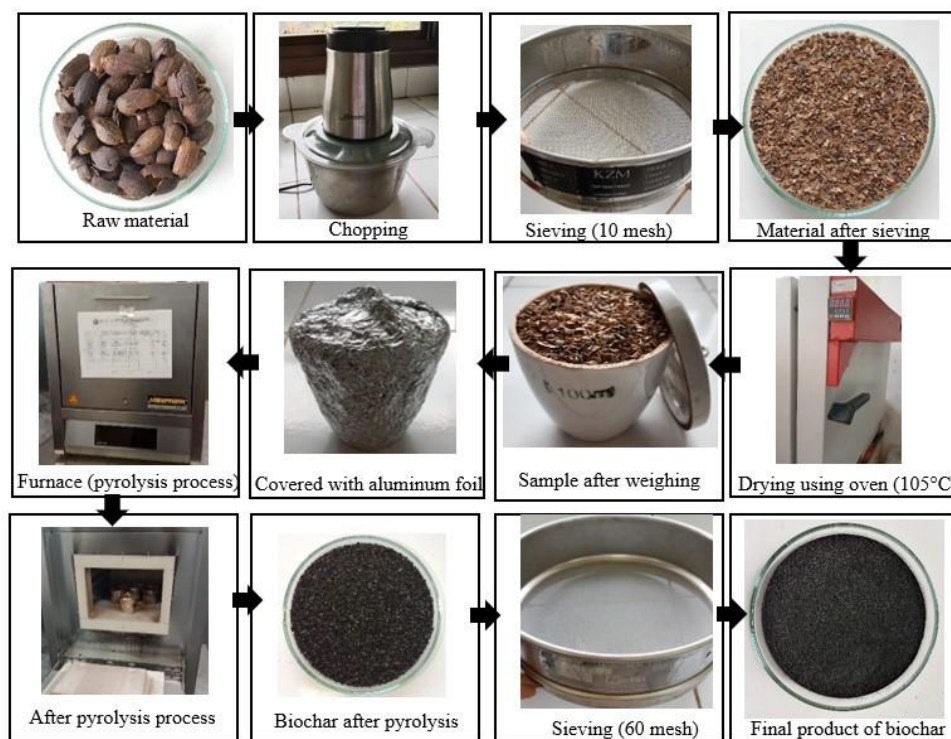
Figure 1. Flowchart of melinjo seed shell biochar production
