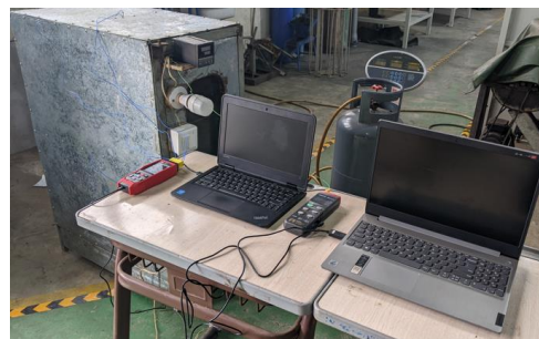
Figure 1. Experimental set-up of the direct gas-fired oven
