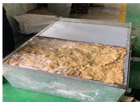
(c) Fiber glass insulation
