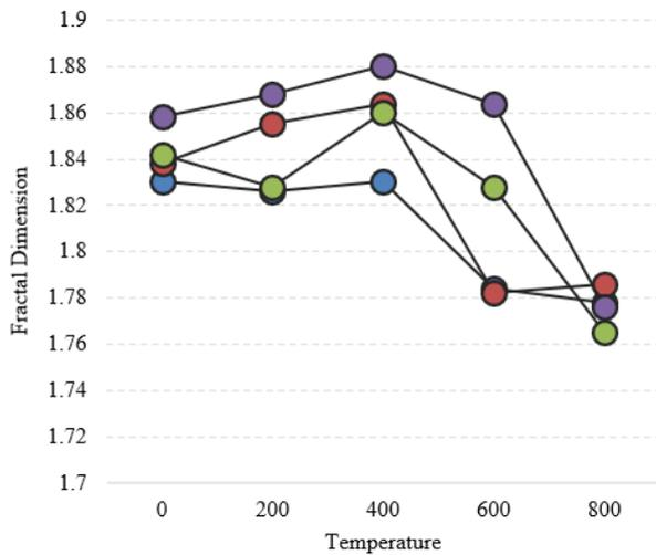
**Figure 3.** Relationship between fractal dimension of concrete and temperature
