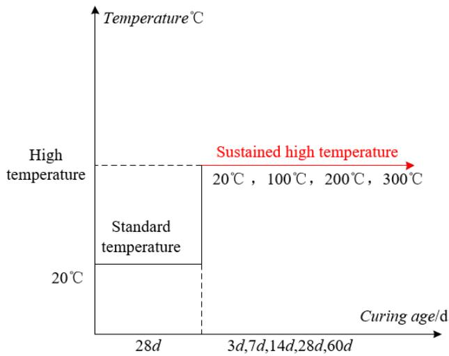
**Figure 2.** Concrete specimen subjected to temperature history for civil engineering use
