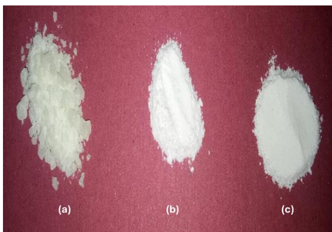
Figure 3. The physical appearance of synthesized HAp with (\text{NH}_4)_2\text{HPO}_4 concentrations of (a) 0.5 M, (b) 1.0 M, and (c) 1.5 M
