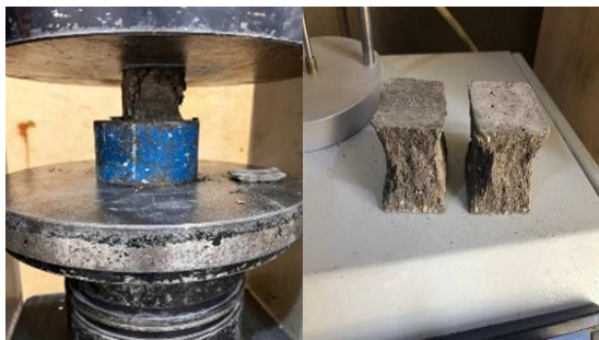
Figure 7. Compressive strength test
