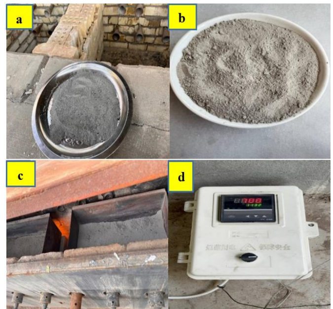
Figure 4. Palm ash: (a) after random burning, (b) after controlled burning, (c) palm ash in the controlled furnace, (d) temperature gauge
