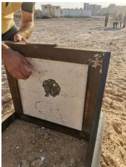
Figure 5. The specimen after gunshots
