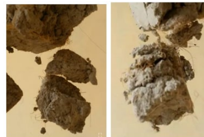
Figure 7. Results of the compression test of paving blocks stored for 6 months
