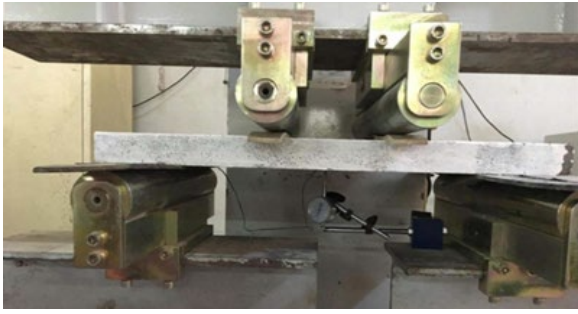
Figure 5. Test setup for flexural test specimen
