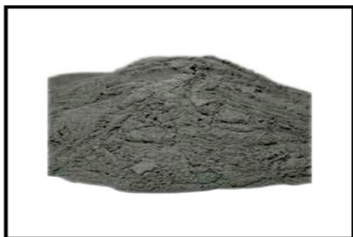
Figure 1. Sieved aluminium dross
