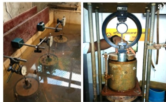
Figure 5. CBR testing setup
