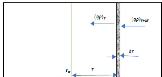
Figure 4. Radial fluid flow near a production well
