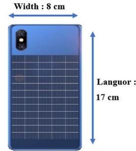
**Figure 6.** Solar panel dimension of a solar DTN node
