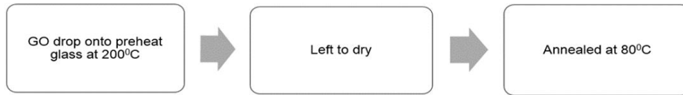
Figure 2. Flowchart illustrating the deposition of graphene thin films using the drop-casting method
