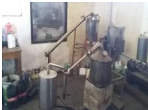
Figure 1. Pyrolysator is a tool that produces liquid smoke
