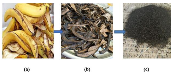
Figure 2. Stages of burning banana peels to adsorbent
