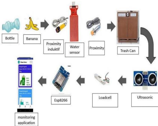
Figure 4. How the system works
