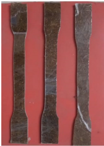
Figure 10. The samples of a composite material made from epoxy resin, Borassus fiber and CBSSP
