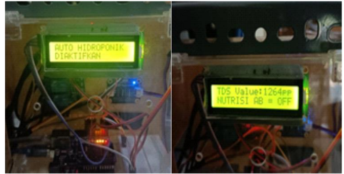
Figure 14. LCD I2C function testing
