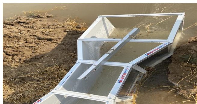
Figure 1. Measuring study area discharge via a Venturi flume
