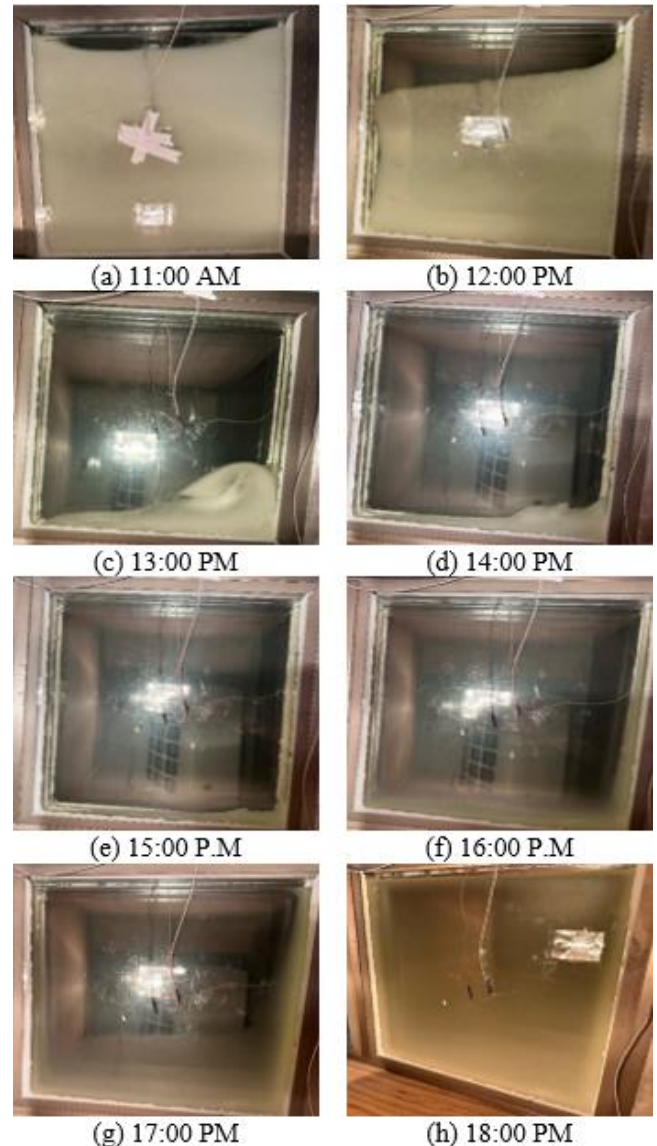
Figure 4. The phase changes of PCM in TG-PCM
