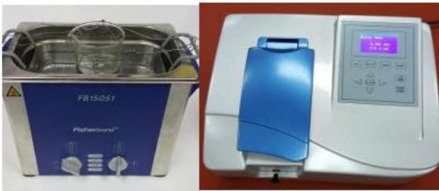
Figure 1. The ultrasonic both vibrator and spectrometer for sonication
