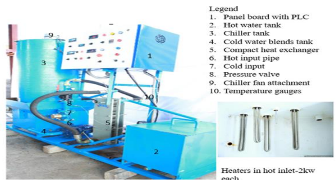
Figure 2. The test-rig setup of compact heat exchanger
