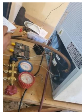
Figure 5. Testing control values for conventional vapour refrigerator
