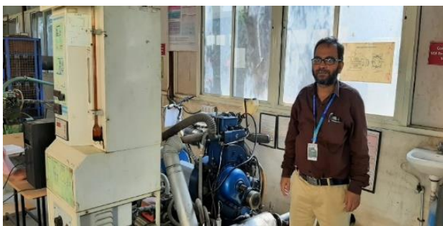
Figure 1. A photographic view of the engine with dynamometer set up
