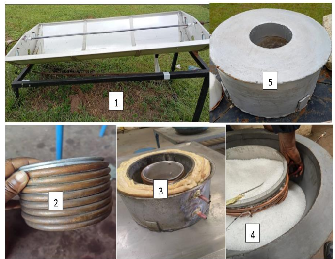
Figure 8. Different components of the final device: 1. Cylindrical-parabolic concentrator, 2. Cooking pot, 3. Heat exchanger, 4. Fiberglass, 5. PCM (phase change material)
