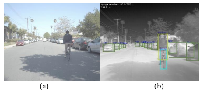
Figure 11. FLIR thermal starter dataset image example (a) RGB visible light image (b) Classification annotated infrared thermal imaging image
