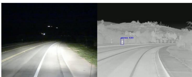
Figure 1. Comparison of RGB image and infrared thermal imager imaging effects under night road conditions
