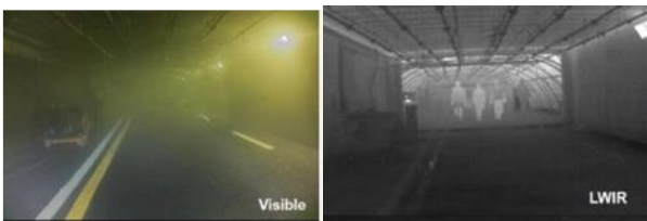
Figure 3. Example images recorded in fog tunnel with thermal (LWIR), visible RGB
