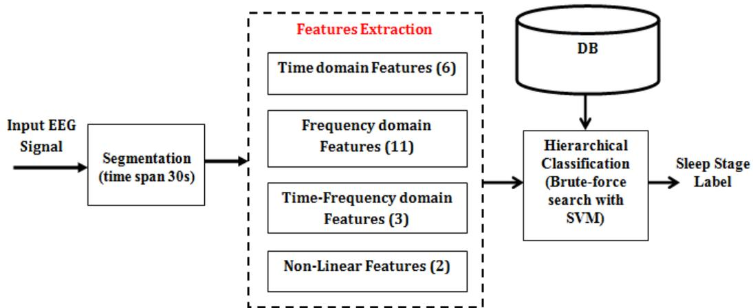
Figure 1. Overall working schematic of proposed sleep staging system
