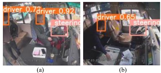
Figure 1. Example of YOLO v5 detection error (a) The model detects multiple drivers; (b) Passengers misclassified as driver
