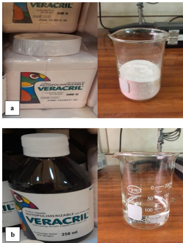
Figure 1. (a) Acrylic resin (PMMA) powder type (Veracril company) and (b) (PMMA) liquid monomer
