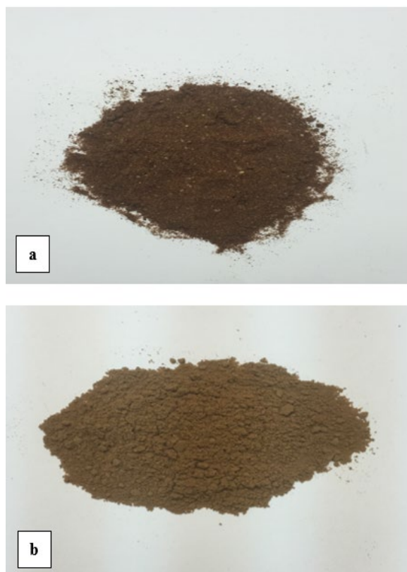
Figure 2. The walnut shells powder used in this study where (a) microparticles size (150µm) and (b) microparticles size (25µm)
